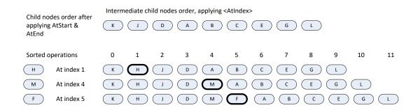
The defined logic also means that if the same xml file is re-ingested a second time, although there may be some internal shuffelling of the elements the final result is the same. As shown in the diagrams below for the same input sequence as above.
